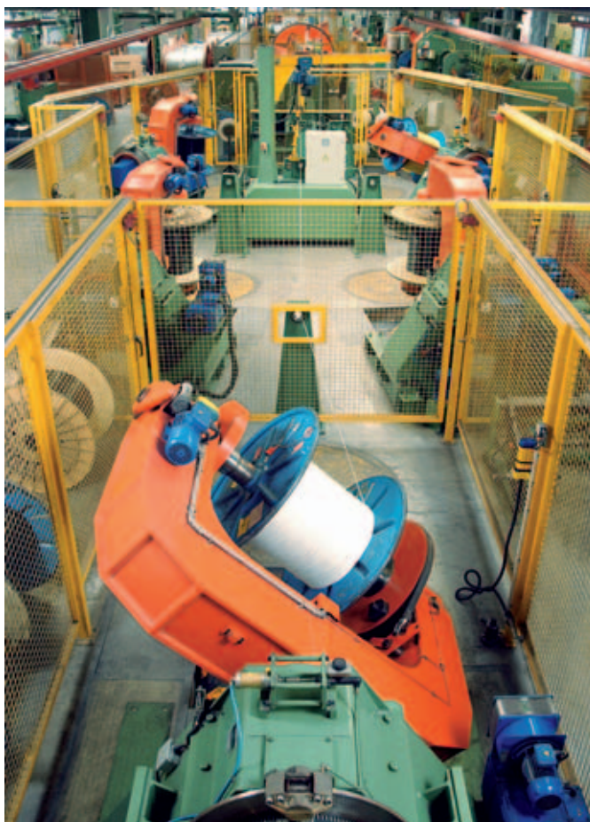
Large cabling machine with backtwist at our Windsbach factory.
